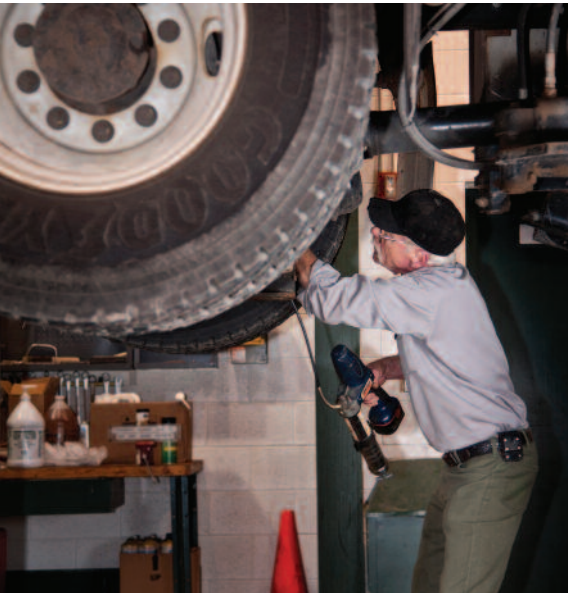
Pictured Rocks National Lakeshore employee William Magli maintains a large snowplow with soy-based lubricants while using a hydraulic lift that also uses soy-based hydraulic fluid.
